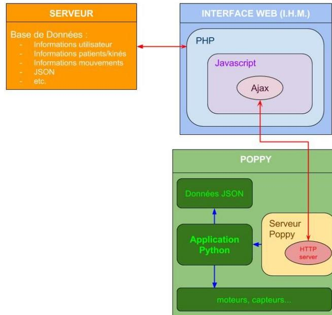
This architecture allows the user to use the application by connecting to the webservice. Consequently, any user can connect to the server from anywhere to use the web interface, and can master any Poppy robot assigned for the application, since he has the access to the server. Moreover, the data are centralised on the web server, that allows every users to have access to up-to-date data without having to manually download them.
