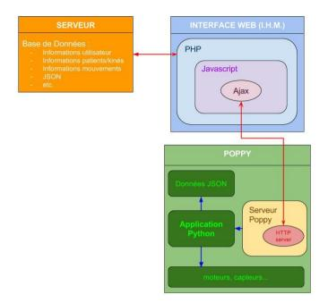
This architecture allows the user to use the application by connecting to the webserver. Consequently, any user can connect to the server from anywhere to use the web interface, and can master any Poppy robot assigned for the application, since he has the access to the server. Moreover, the data are centralised on the web server, that allows every users to have access to up-to-date data without having to manually download them.
