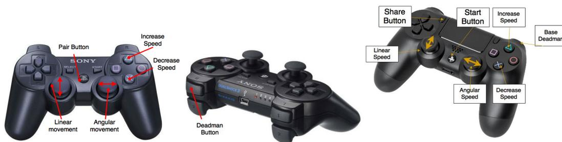
Figure 2 – Base Operation Mode for PS3 and PS4 pads
