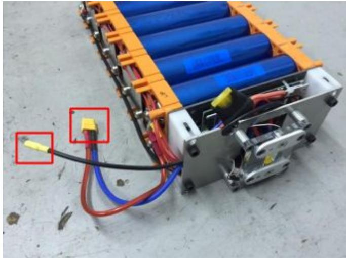
Figure 21– Power supply connector from the Battery Pack
