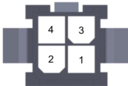
Figure 39 - Molex pinout
