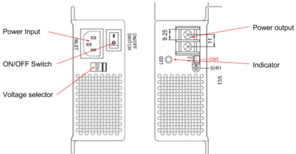
Figure 25– Charger connections
