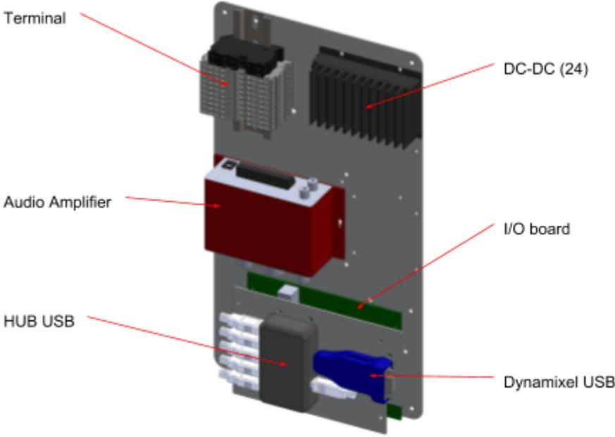
Figure 33 – Interior torso components
