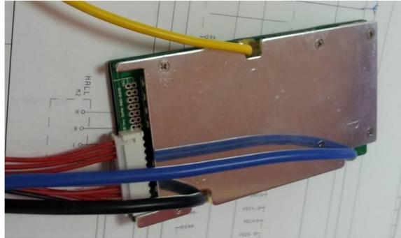
Figure 23– Protection circuit module
