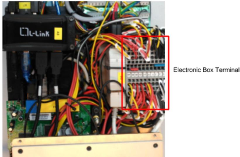
Figure 10- Electronic box terminal location
