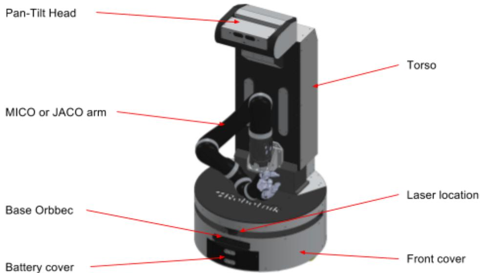
*Figure 1 – Front view of RB-1 robot*
