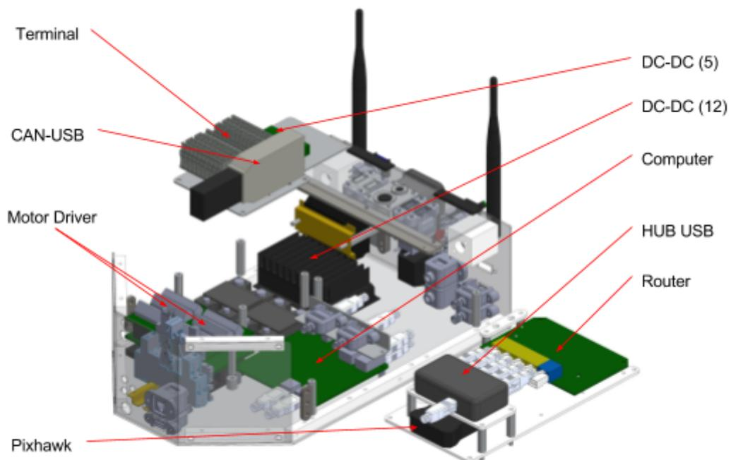
Figure 30 – Electronic box components
