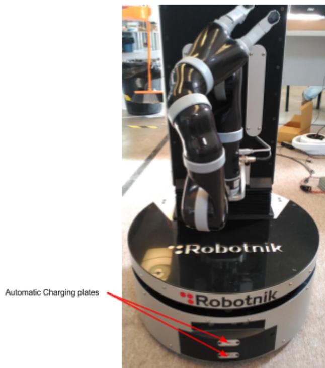
Figure 18- Plates for automatic charge
