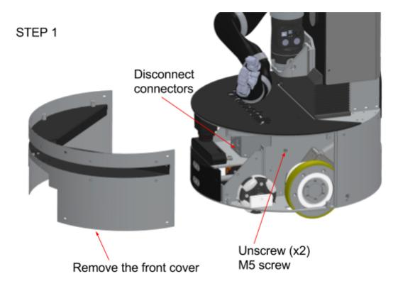
Figure 28 - Electronic box extraction - Step 1
