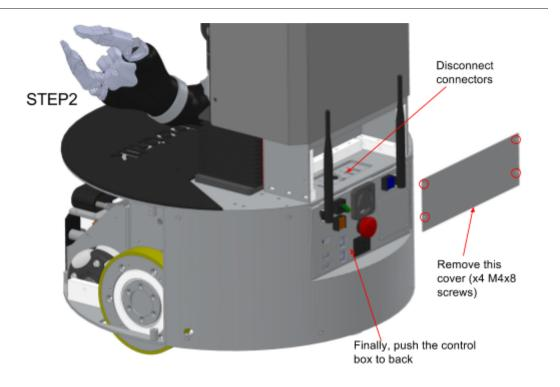
Figure 29 – Electronic box extraction - Step 2
