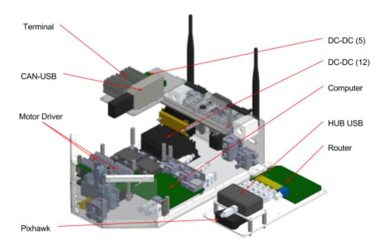
Figure 30 – Electronic box components
