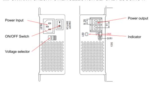
Figure 25- Charger connections
