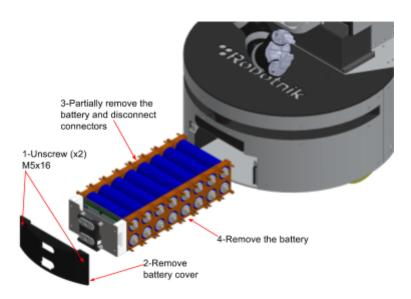
Figure 36- Battery pack removal
