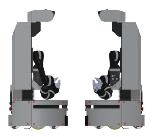
Figure 26 - Front and back cover screw removal
