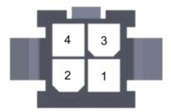
Figure 39 - Molex pinout
