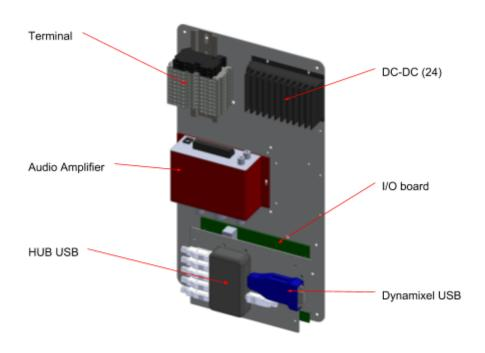
Figure 33 – Interior torso components
