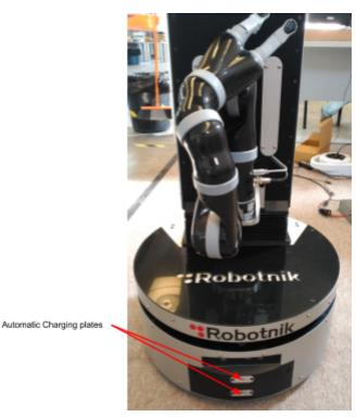
Figure 18- Plates for automatic charge
