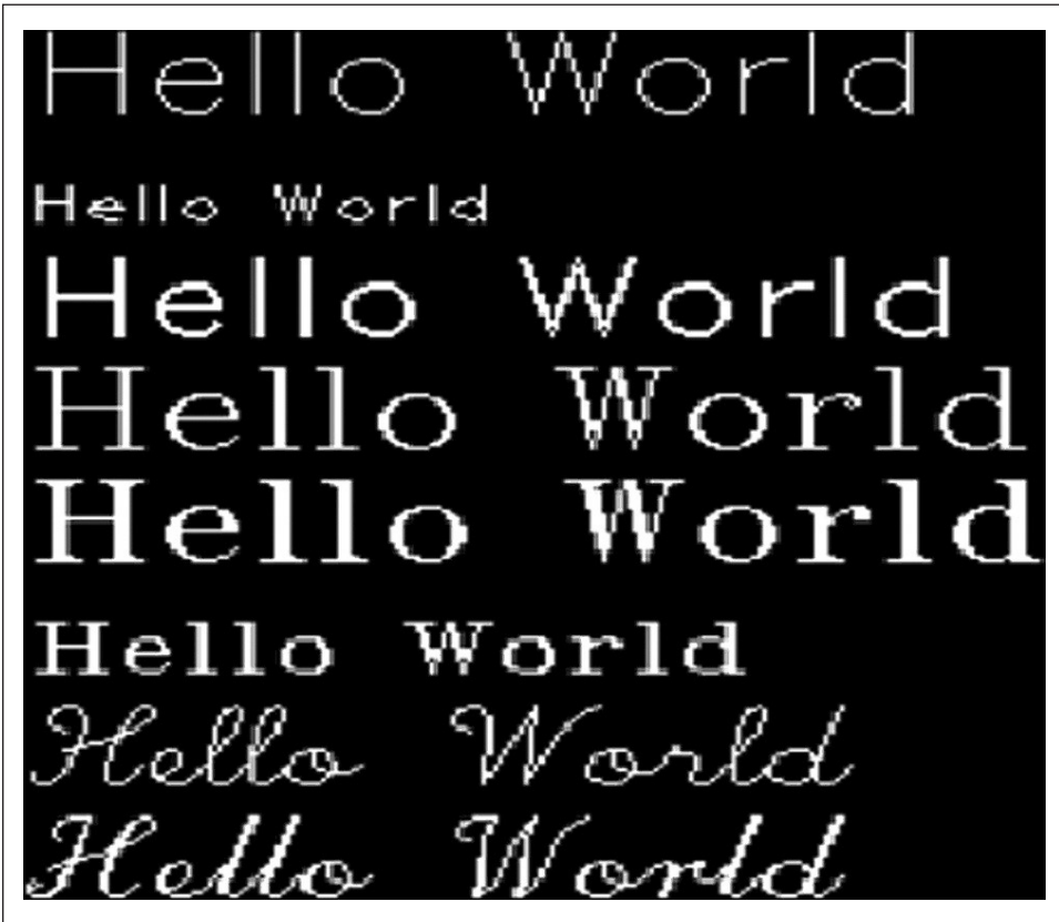
Figure 3-6. The eight fonts of Table 3-15 drawn with h_{scale} = v_{scale} = 1.0 , with the origin of each line separated from the vertical by 30 pixels
