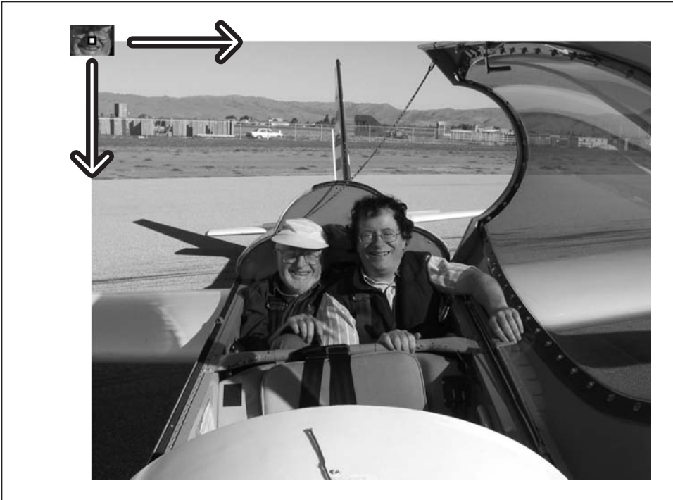
Figure 7-10. cvMatchTemplate() sweeps a template image patch across another image looking for matches
