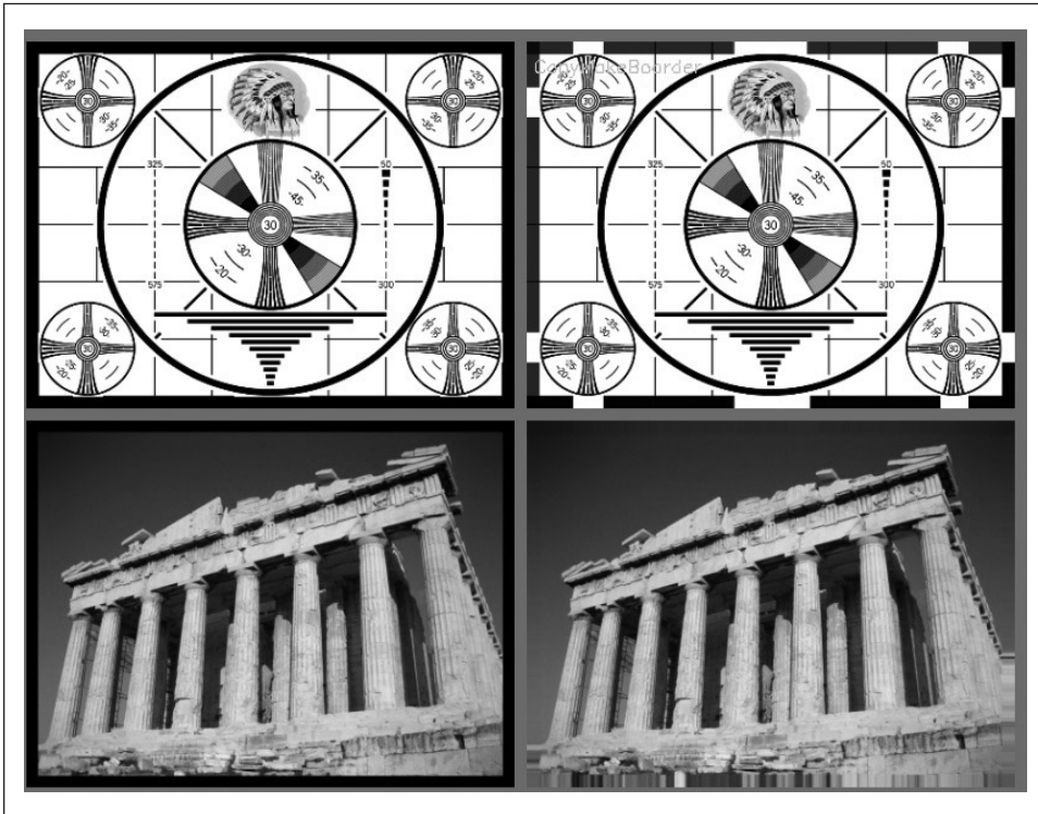
Figure 6-2. Expanding the image border. The left column shows IPL_BORDER_CONSTANT where a zero value is used to fill out the borders. The right column shows IPL_BORDER_REPLICATE where the border pixels are replicated in the horizontal and vertical directions
