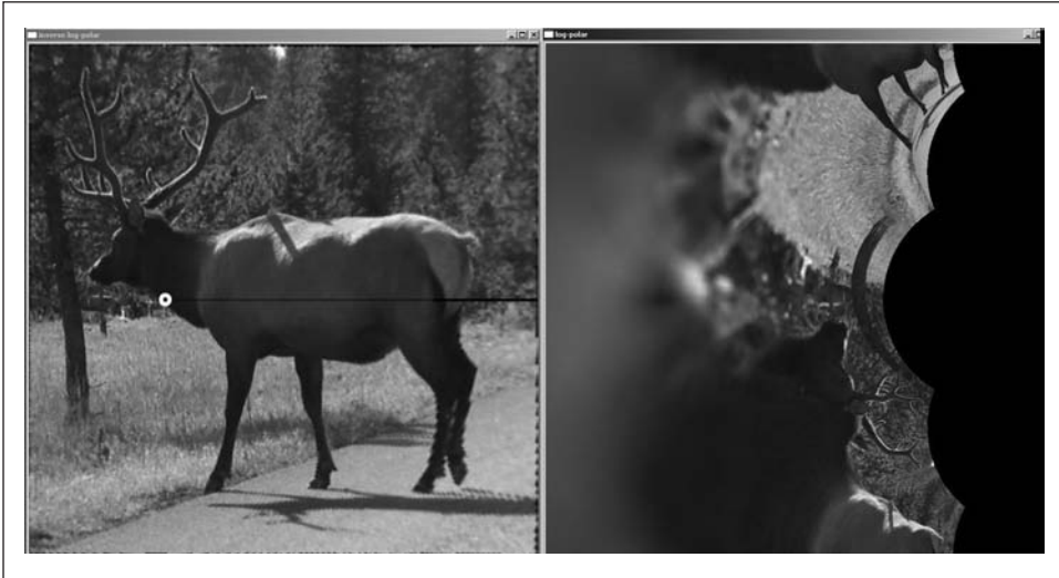
Figure 6-17. Log-polar example on an elk with transform centered at the white circle on the left; the output is on the right
